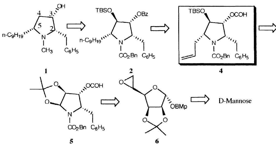
The key step is the Lewis acid-promoted addition of allyltrimethylsilane to the bicyclic ketal **5** to introduce the correct R configuration at C5.
